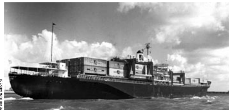
ABOVE: Converted from a C5 cargo ship, Sealand's Gateway City made her first voyage as a fully-cellular container ship in late 1957 when she carried 226 35ft containers between New Jersey and Miami.
